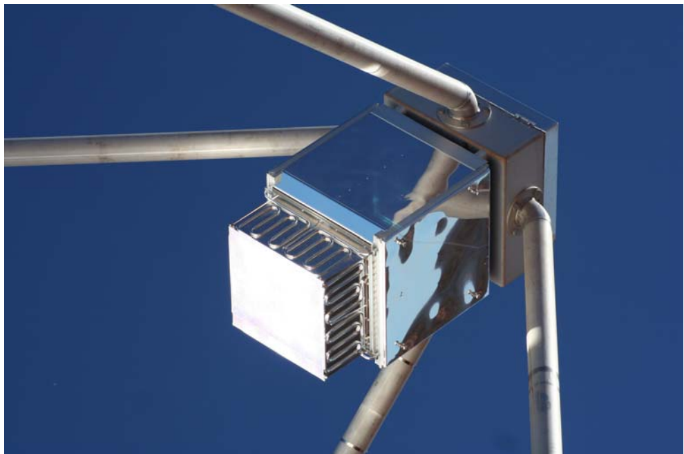
30% efficiency receiver 'on-sun' at Hermannsburg
