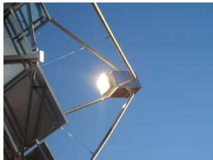
World record solar PV receiver generating electricity from concentrated sunlight in a solar dish in Central Australia
